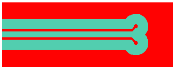
Differential impedance lines, with AOI pad in \text{aoi\_pad\_dx} > 0 & \text{aoi\_pad\_dy} > 0
