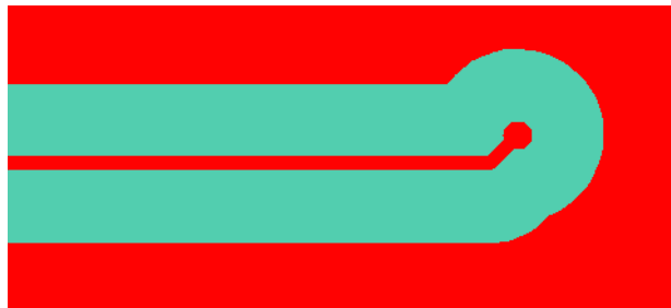
Single ended impedance line, with AOI pad in a \text{aoi\_pad\_dx} > 0 & \text{aoi\_pad\_dy} > 0
